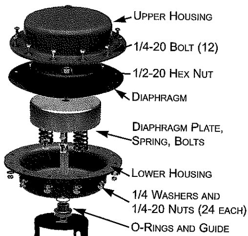
Figure 7-DIAPHRAGM REMOVAL (Direct Acting)
